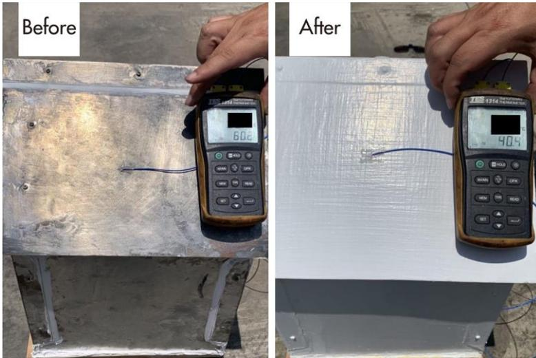
Applying M168 can reduce exterior temperature up to 20 degrees.
